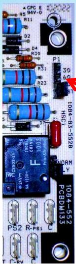
Install jumper wire across test terminals of control board.
